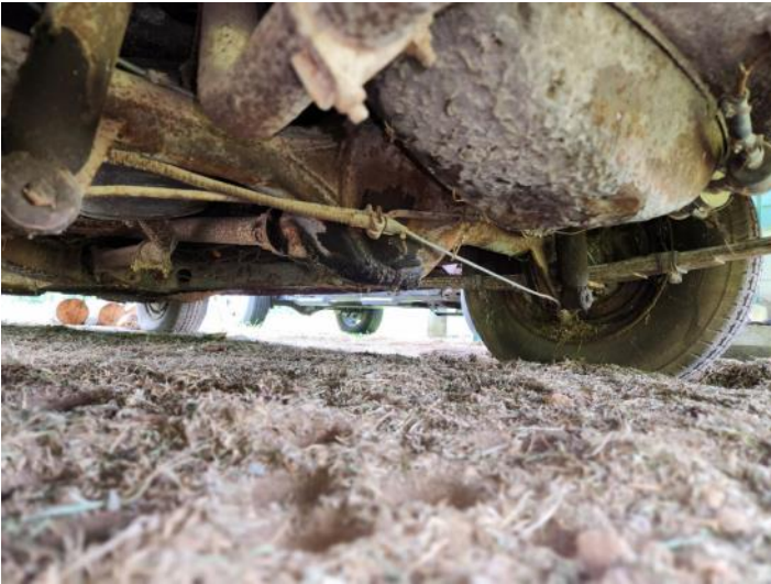
Old Ruby's faulty emergency brake setup
