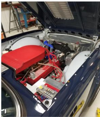
Above, the sleeper TR6 with its Rover V8 engine.
