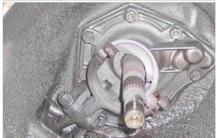
Top, throw-out bearing; bottom, clutch fork.
