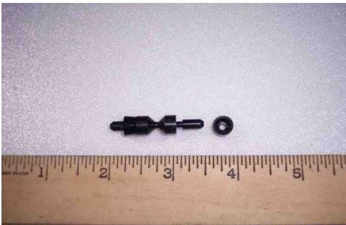
Proportioning valve (cup-type)
